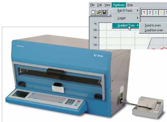
temp-gard temperature data is transferred to gradient-oven.
