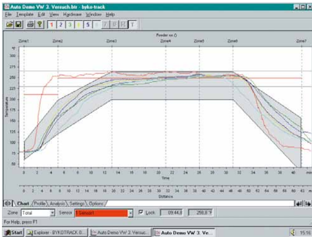
temp-gard collects temperature data in production oven.
