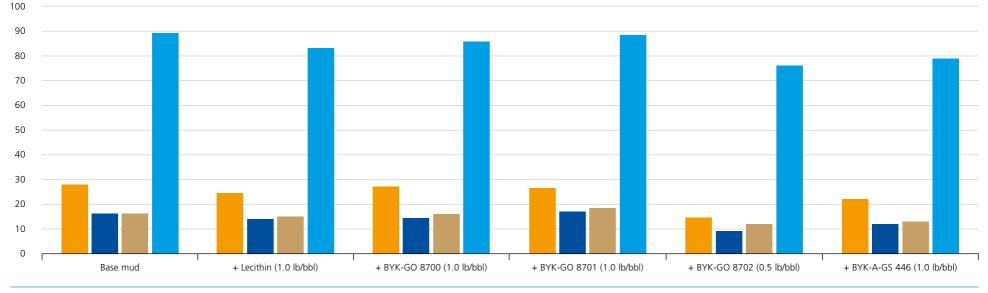
The muds were hot rolled at 250 °F for 16 hours and tested again at 150 °F. BYK-GO 8700 and BYK-GO 8701 both performed equally as well as lecithin. At 250 °F, BYK-GO 8702 and BYK-A-GS 446 again conditioned the mud to optimal rheological ranges.
