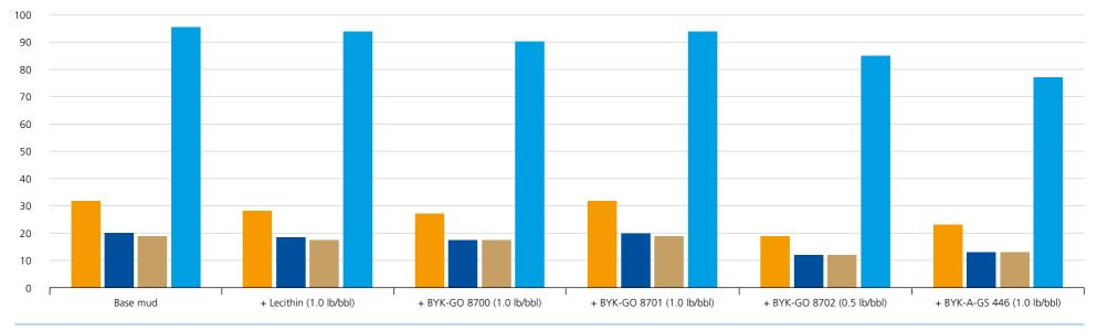
The drilling fluids were additionally heat-aged at 350 °F for 16 hours. Following the same procedure, rheological data were collected at 150 °F. After heat aging at this temperature, BYK-GO 8700, BYK-GO 8701, BYK-GO 8702 and BYK-A-GS 446 were found to be efficient thinners, each exhibiting temperature stability at 350 °F. The yield point, 6-rpm rheology, and 30-minute gel strength were consistent for each of the products.
