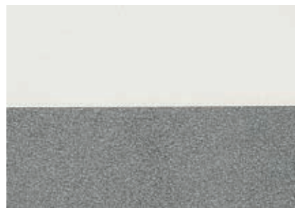
Without Air Release Additive
