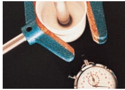
Using a Dispermat for 30 seconds
