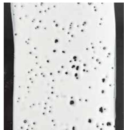
Poor mold surface wetting because of gel coat's high surface tension.
