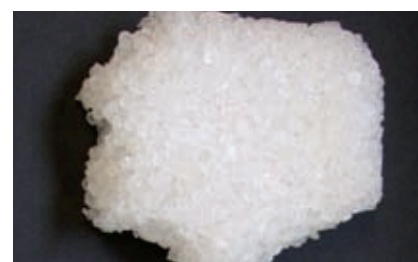
Granules after being stored for 1 hr at 70 °C/158 °F in an oven
