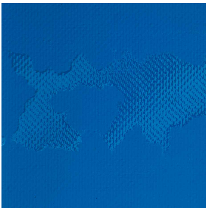
Poor substrate wetting of an aqueous coating on PVC foil
