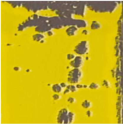
Poor substrate wetting on oily substrate
