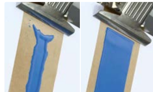
Insufficient wetting without surface additive
