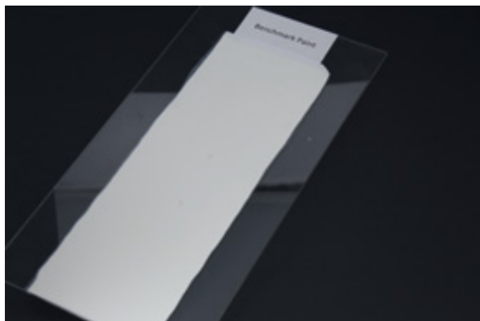
Figure 6: Sample plate with applied wall paint without scuffing (good).
