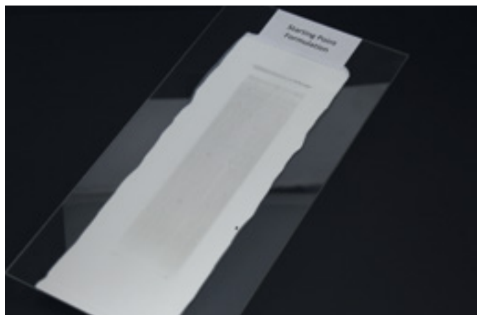
Figure 7: Sample plate with applied wall paint with scuffing (bad).
