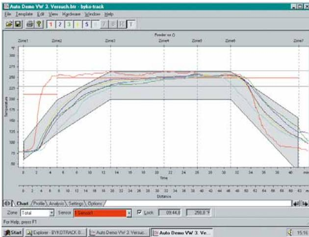
The temp-gard system controls the curing process and immediately evaluates the results. Within a few minutes all important information is available on the screen and can be printed out:
