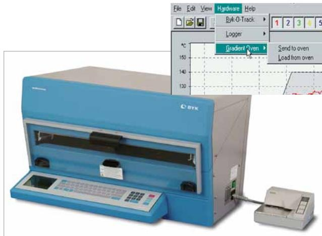
temp-gard temperature data is transferred to gradient-oven.
