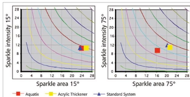
BYK-mac measurement data correlates with a visual judgment. The sparkle area for the system with wax additive at 75° is smaller than for the two other systems. As Sparkle 75° evaluates flakes which are non-parallel oriented, this clearly shows that by using the BYK-Chemie wax additive AQUATIX® the orientation of the aluminum flakes is improved.
