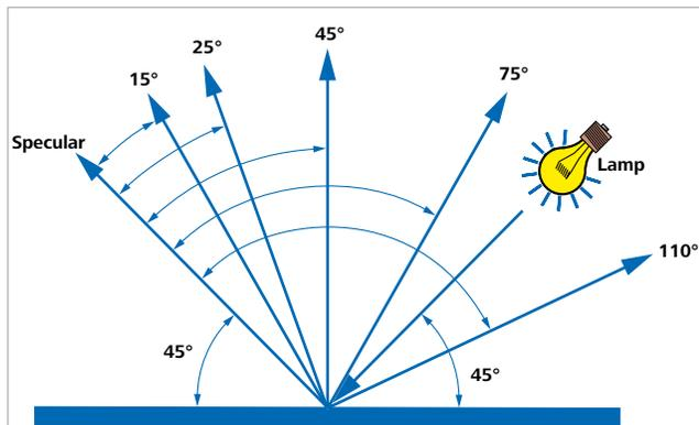
Directional illumination is used versus circumferential illumination because circumferential illumination minimizes the contribution from directional effects such as the Venetian blind effect and surface irregularities. Thus, averaging of the circumferential illumination would cause the measured color values of two specimens to be the same, while visually the two specimens would not match.
