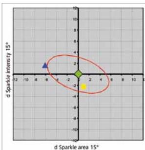
In order to set visually acceptable limits a new sparkle tolerance model was developed together with several partners from the automotive, pigment and paint industry. As a guideline the weighted total color difference equations were used resulting in an elliptical tolerance model.
