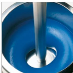
This laminar flow pattern is obtained when the diameter for the vessel and the impeller as well as the distance between plane of disc and base of vessel are matched to one another.
