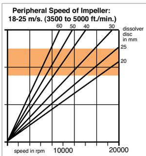
Example: If an impeller disc of 30 mm diameter is used, the Dispermat® must be run at a rotational speed of 10,000 to 15,000 rpm to obtain peripheral velocities of 18 to 25 m/s (3000 ft/min to 5000 ft/min) which is used in many production applications.
