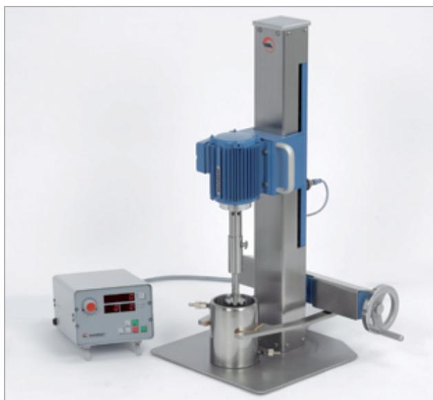
The best dispersion results are obtained with the highest possible mechanical power input without destroying the so called "doughnut" flow pattern.
