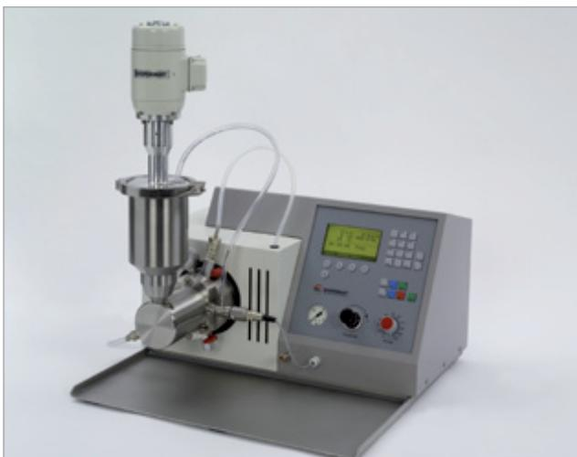
The actual dispersing system consists of a chamber and a rotor; the chamber is filled with grinding media and the product to be dispersed. The actual particle size reduction is accomplished by the moving grinding material, which is activated by a high speed and high energy agitator.
