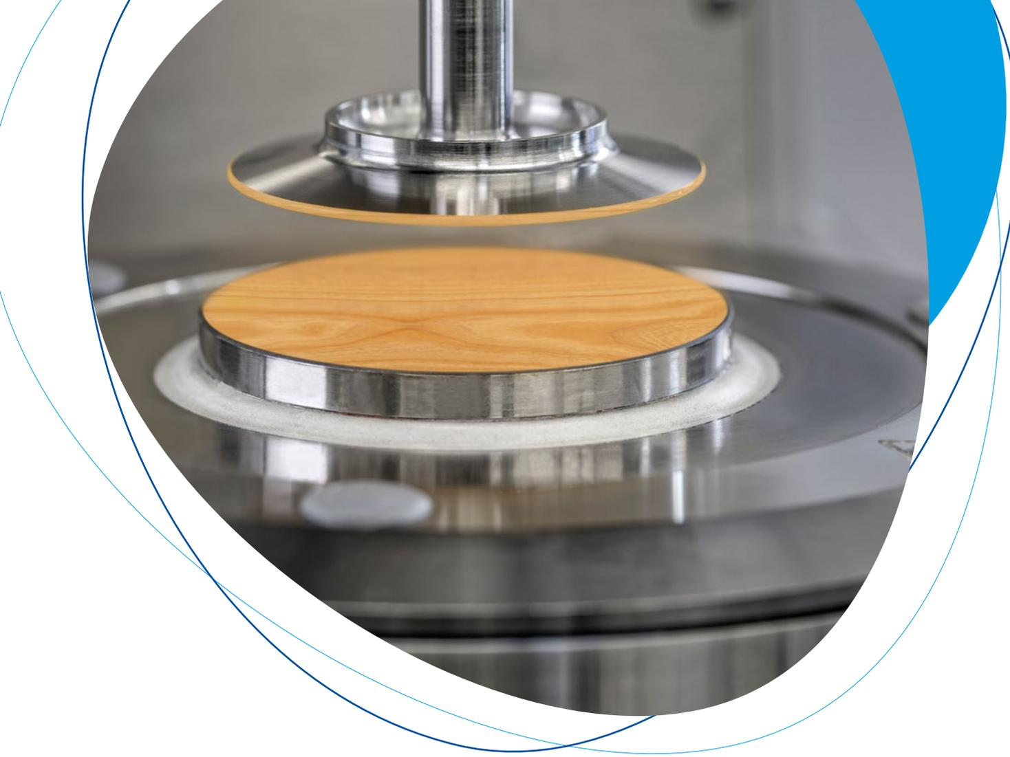
A circular inset image showing a rheology test. A wooden disc is mounted on a metal base, and a metal plate is positioned above it, ready to be lowered. The setup is part of a larger machine, likely a rheometer, used for testing the flow properties of coatings.
