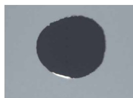
Reduction of the surface tension using a silicone-based additive: better substrate wetting
